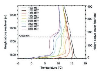
Fig. 10. Selected tethersonde soundings from the center of the crater floor illustrating temperature profile evolution during the evening of 22 Oct. Sounding times are given in the legend.
